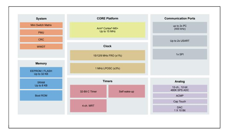
View additional information for LPC800: 32-Bit Arm® Cortex®-M0+-Based Low-Cost MCU.
