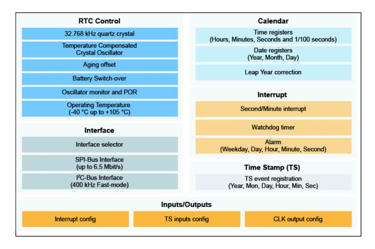
View additional information for Nano-Power Highly Accurate RTC with Integrated Quartz Crystal for Automotive Applications.
