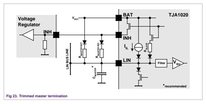
The resistors  $R_{MASTER-BAT}$  and  $R_{MASTER-INH}$  in parallel determine the master termination while the TJA1020 is in its modes: Standby, Normal-slope and Low-slope. In Sleep mode the master termination is determined by  $R_{MASTER-BAT}$ . Therefore the maximum LIN bus short-circuit current  $I_{SC,max}$  can be trimmed by  $R_{MASTER-BAT}$ :
