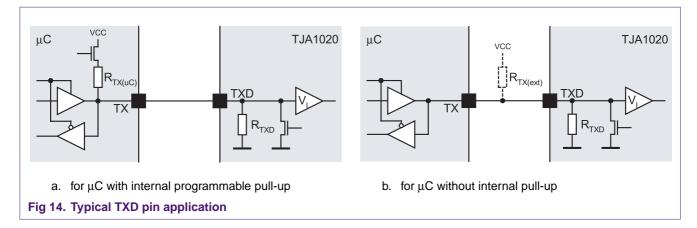
The open drain output as well as the maximum value of the input threshold  $V_{IH(TXD)}$  (Ref. 1) are designed to support 3.0 V/3.3 V as well as 5 V microcontroller derivatives. Thus 3.0 V/3.3 V microcontroller derivatives without 5 V tolerant ports can be used for the TJA1020.
