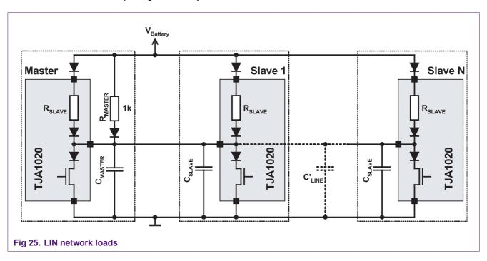
In a LIN network the master resistor  $R_{MASTER}$  (Ref. 2) and the slave resistors  $R_{SLAVE}$  (Ref. 2) are accurately defined by the LIN standard (Ref. 2). No variation is allowed. Also the specified slave capacitance  $C_{SLAVE}$  (Ref. 2) provides almost no room for network optimizations. Only the master capacitor  $C_{MASTER}$  (Ref. 2) can be used to tune the LIN bus signal in either way.
