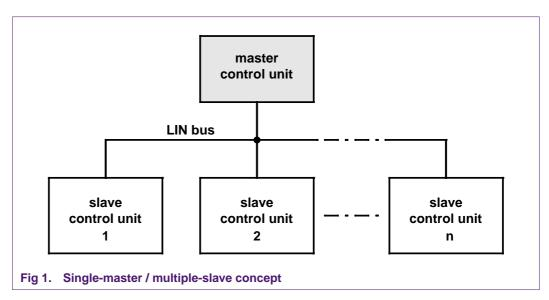
The LIN protocol (Ref. 2) is based on the UART/SCI serial data link format using 8N1-coded byte fields. A LIN network consists of one master node and one or more slave nodes; the medium access is controlled by the master node. Such a single-master/multiple-slave concept is shown in Figure 1.
