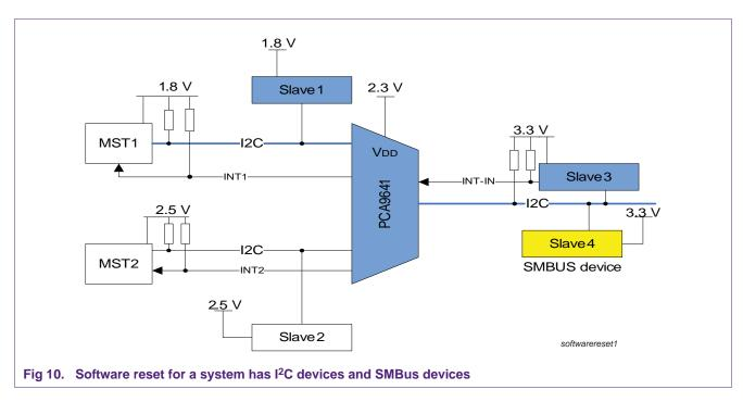
Slave4 is a SMBus slave device, it will not reset when general call software reset is sent. If SMBUS\_WSRST is set, PCA9641 will send SMBus time-out (35 ms SCL low) and then reset PCA9641.
