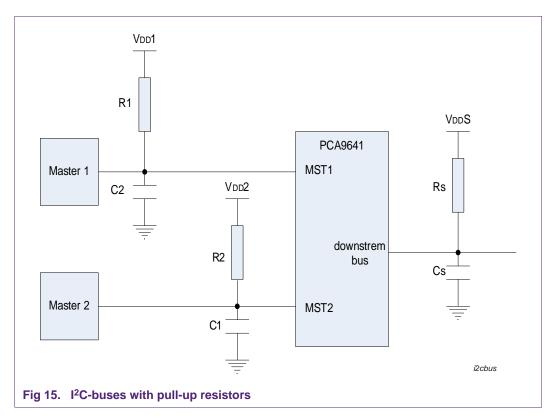
PCA9641 provides isolation between two masters but do not provide any additional drive capability or isolate capacitance between the master buses and downstream bus. Therefore, the overall capacitance of the highest master bus and downstream bus must be taken into consideration when choosing the value of pull-up resistor.
