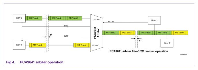
A transaction includes many  $I^2C$  start conditions and stop conditions and idle times. Note: idle time should not be longer than 100 ms.
