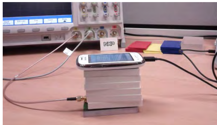
Fig 15. Recommended approach to spy RF activity
