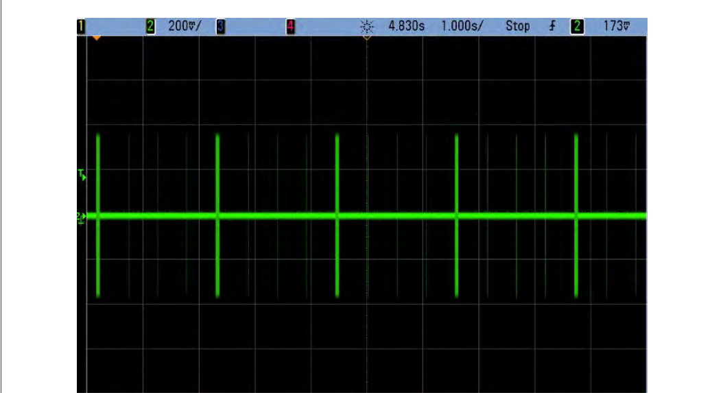
Fig 7. Oscilloscope screenshot of Hybrid mode with POLL phase every 3 LPCD pulses @ 2Hz
