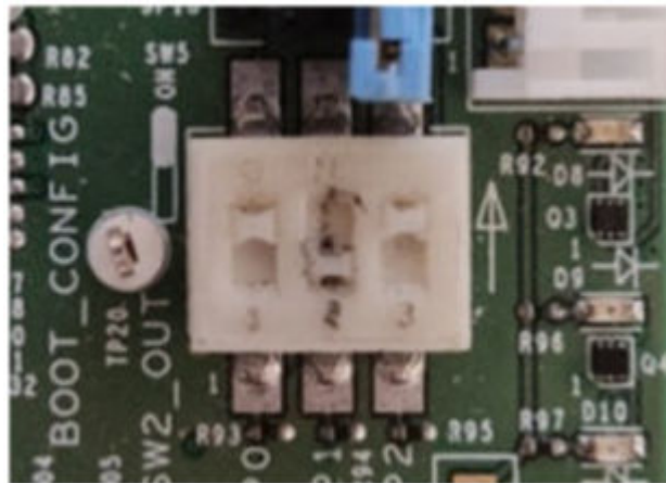
Figure 21. Setting SW5 to 1-ON, 2-OFF, 3-ON
