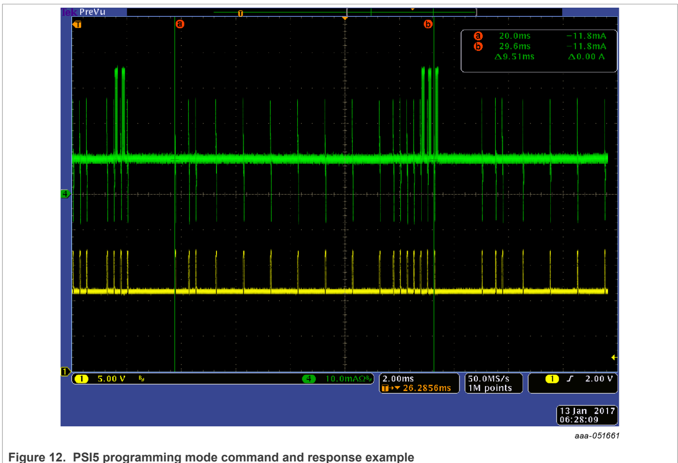
Figure 11. PSI5 programming mode write register command and response format
