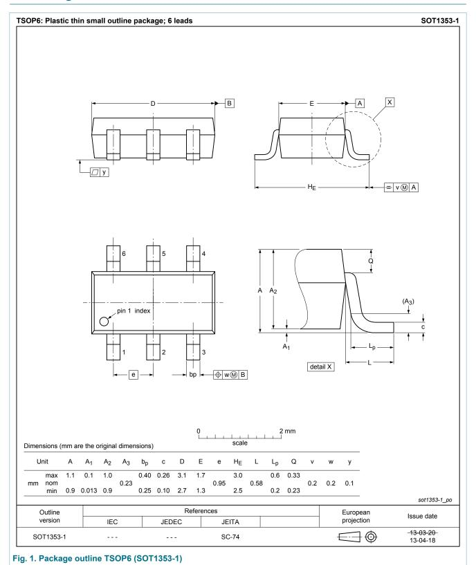
plastic surface-mounted package (TSOP6); 6 leads
