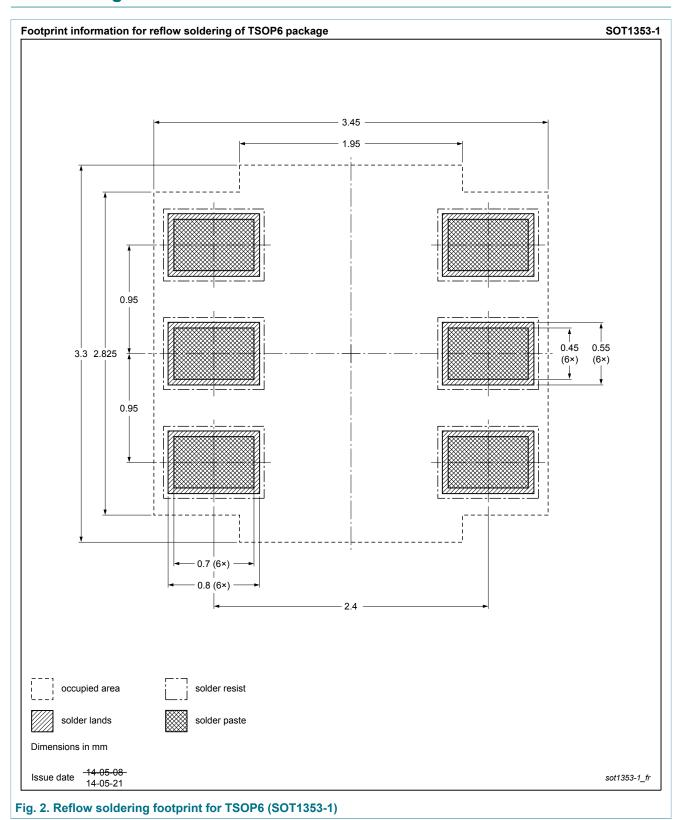
plastic surface-mounted package (TSOP6); 6 leads
