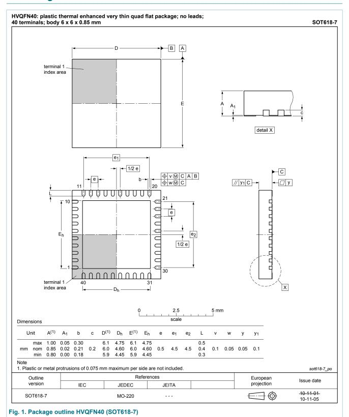
plastic thermal enhanced very thin quad flat package; no leads; 40 terminals
