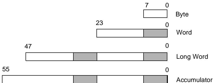
Figure 12-3. Operand Lengths in Sixteen-Bit Mode
