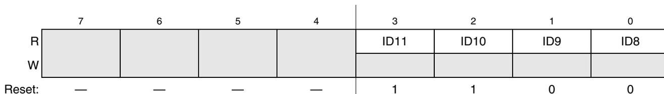
Figure 5-5. System Device Identification Register — High (SDIDH)
