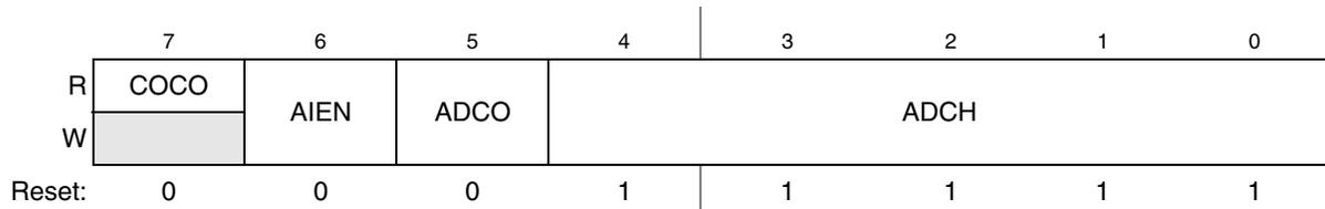
**Figure 9-2. Status and Control Register (ADCSC1)**
