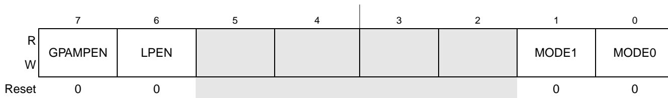
Figure 19-3. GPAMP Control Register 0 (GPAMPxC0)
