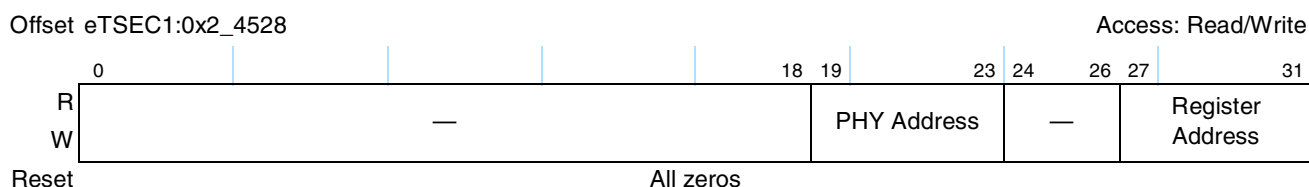
Figure 18-42. MIIMADD Register Definition
