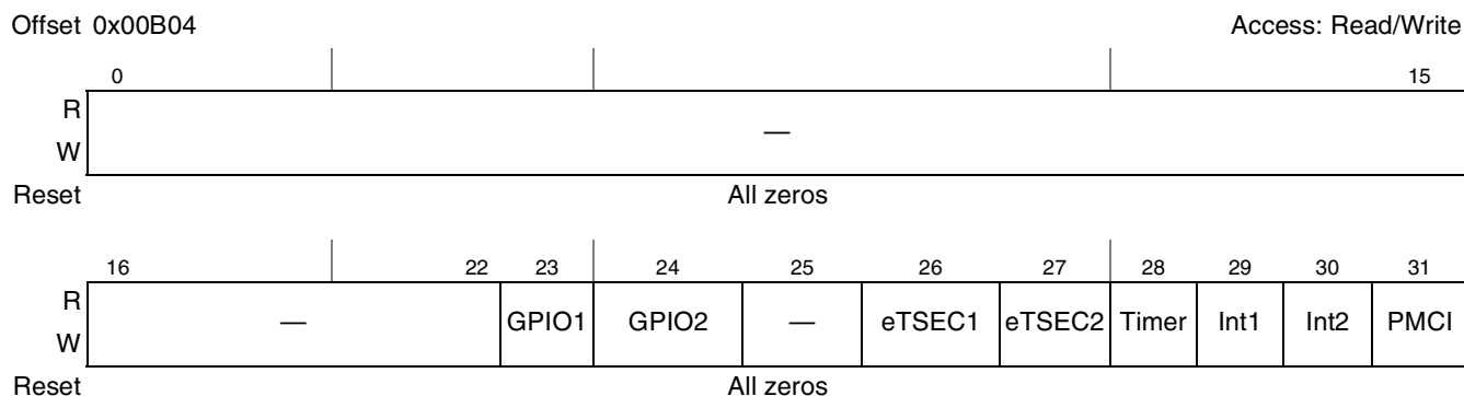
Figure 5-58. Power Management Controller Event Register
