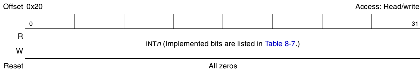
Figure 8-10. System Internal Interrupt Mask Register (SIMSR_H)
