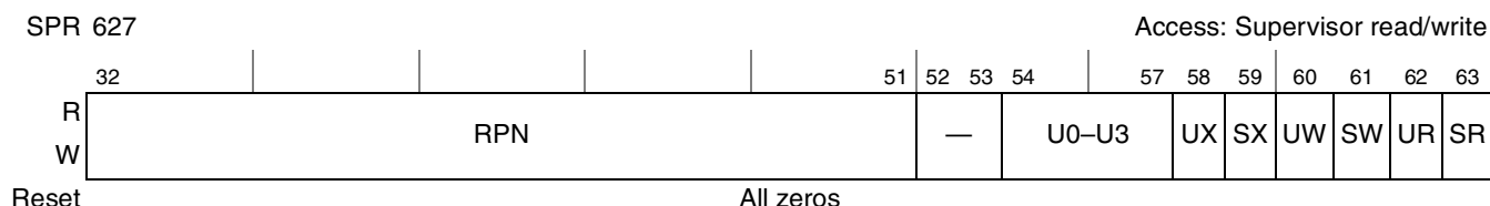
Figure 6-46. MAS Register 3 (MAS3)
