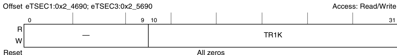
Figure 15-56. Transmit and Received 512- to 1023-Byte Frame Register Definition
