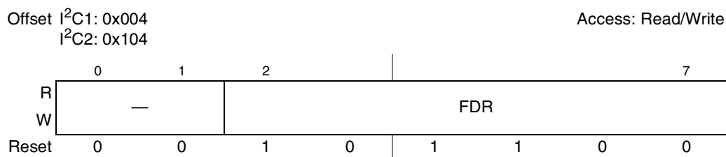
Figure 11-3. I 2 C Frequency Divider Register (I2CFDR)
