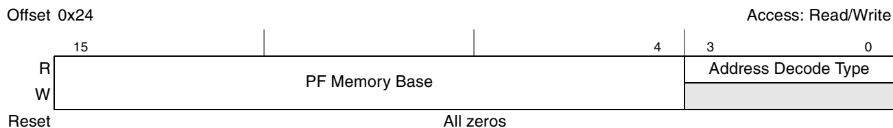
Figure 18-68. PCI Express Prefetchable Memory Base Register
