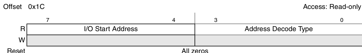
Figure 18-63. PCI Express I/O Base Register
