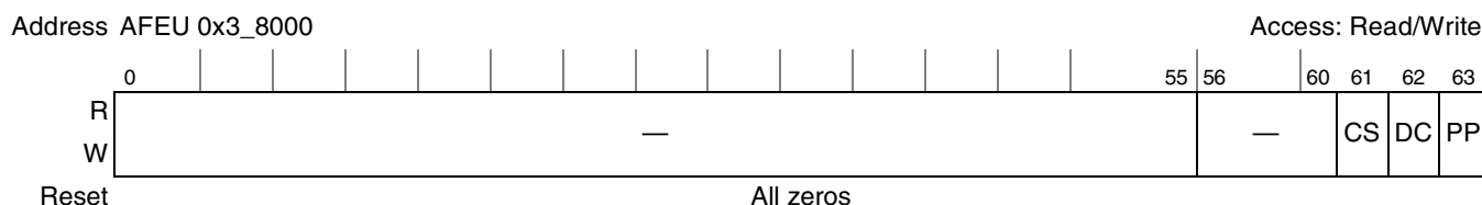
Figure 12-21. AFEU Mode Register
