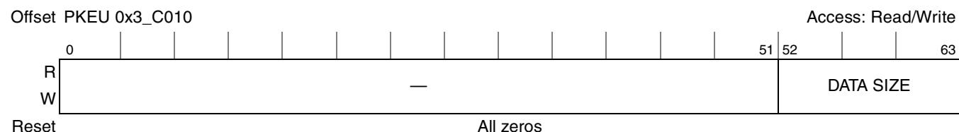
Figure 12-10. PKEU Data Size Register
