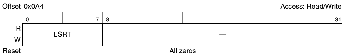
Figure 14-12. LSRT SDRAM Refresh Timer (LSRT)
