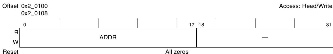
Figure 7-11. L2 Memory-Mapped SRAM Base Address Registers (L2SRBAR n )
