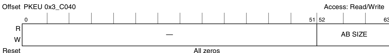
Figure 12-9. PKEU AB Size Register
