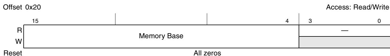
Figure 18-66. PCI Express Memory Base Register
