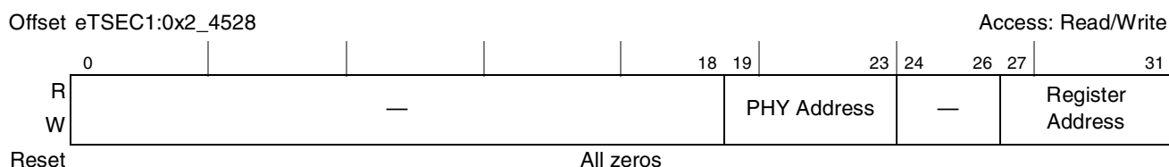
Figure 15-43. MIIMADD Register Definition
