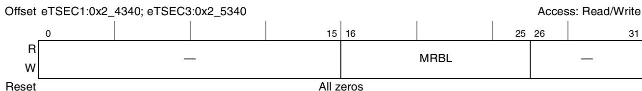
Figure 15-31. MRBLR Register Definition
