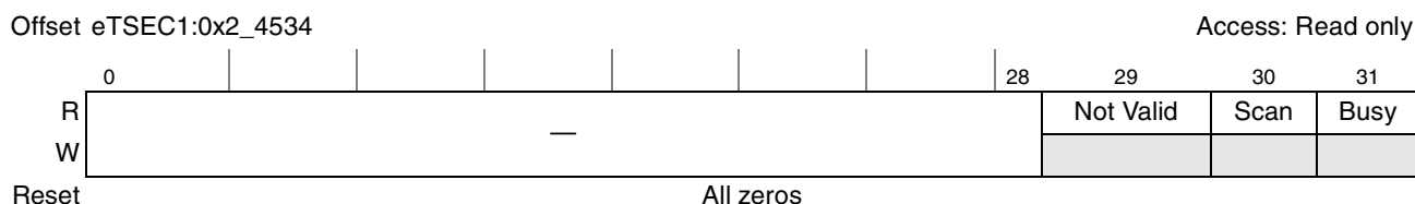
Figure 15-46. MII Mgmt Indicator Register Definition
