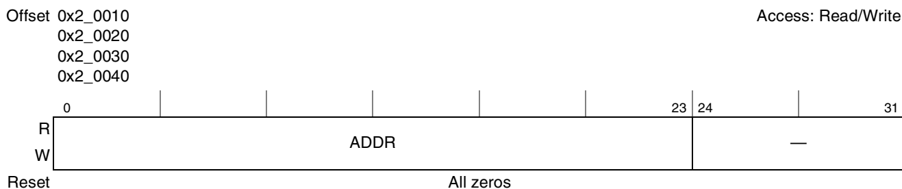
Figure 7-8. Cache External Write Address Registers (L2CEWAR n )
