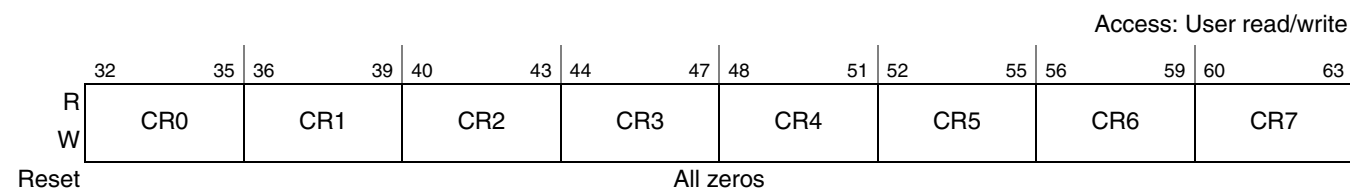
Figure 6-3. Condition Register (CR)
