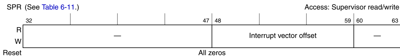
Figure 6-21. Interrupt Vector Offset Registers (IVOR n )
