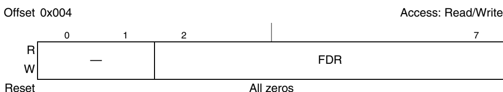
Figure 11-3. I 2 C Frequency Divider Register (I2CFDR)
