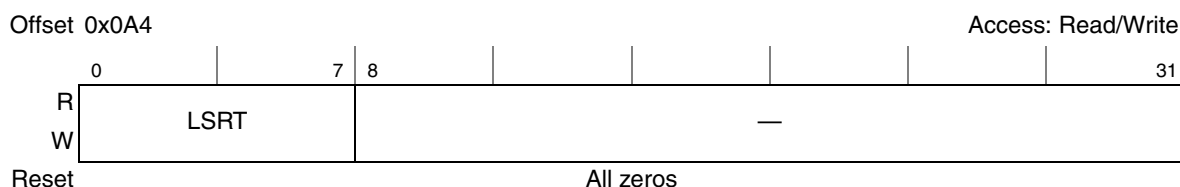
Figure 13-12. LSRT SDRAM Refresh Timer (LSRT)
