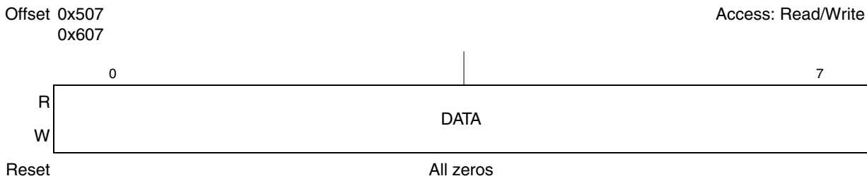
Figure 12-13. Scratch Register (USCR)
