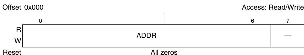
Figure 11-2. I 2 C Address Register (I2CADR)
