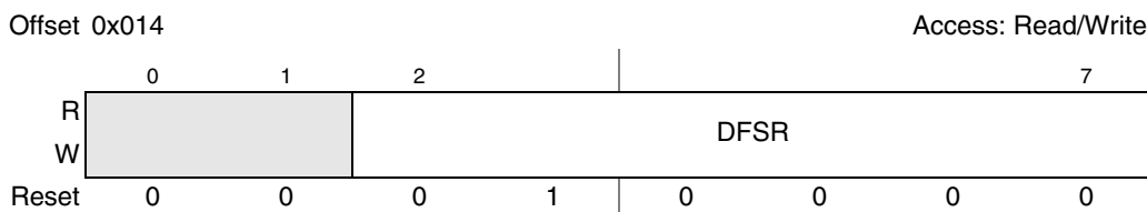
Figure 11-7. I 2 C Digital Filter Sampling Rate Register (I2CDFSRR)
