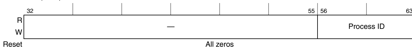
Figure 6-37. Process ID Registers (PID0–PID2)
