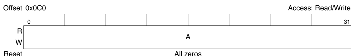
Figure 13-17. Transfer Error Address Register (LTEAR)
