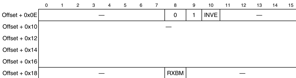
Figure 41-30. AAL0 Protocol-Specific RCT
