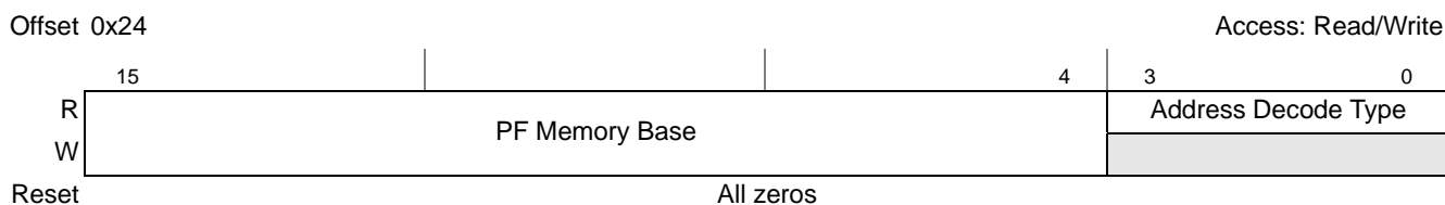
Figure 17-79. PCI Express Prefetchable Memory Base Register
