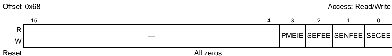
Figure 17-105. PCI Express Root Control Register
