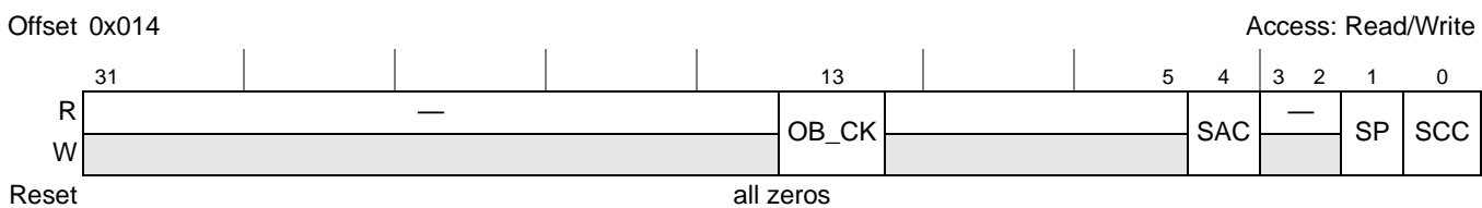
Figure 17-16. PCI Express Configuration Register (PEX_CONFIG)
