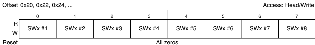
Figure 44. Switch Registers (PX_SWx)
