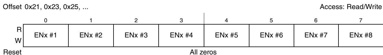
Figure 45. Switch Enable Register (PX_ENx)
