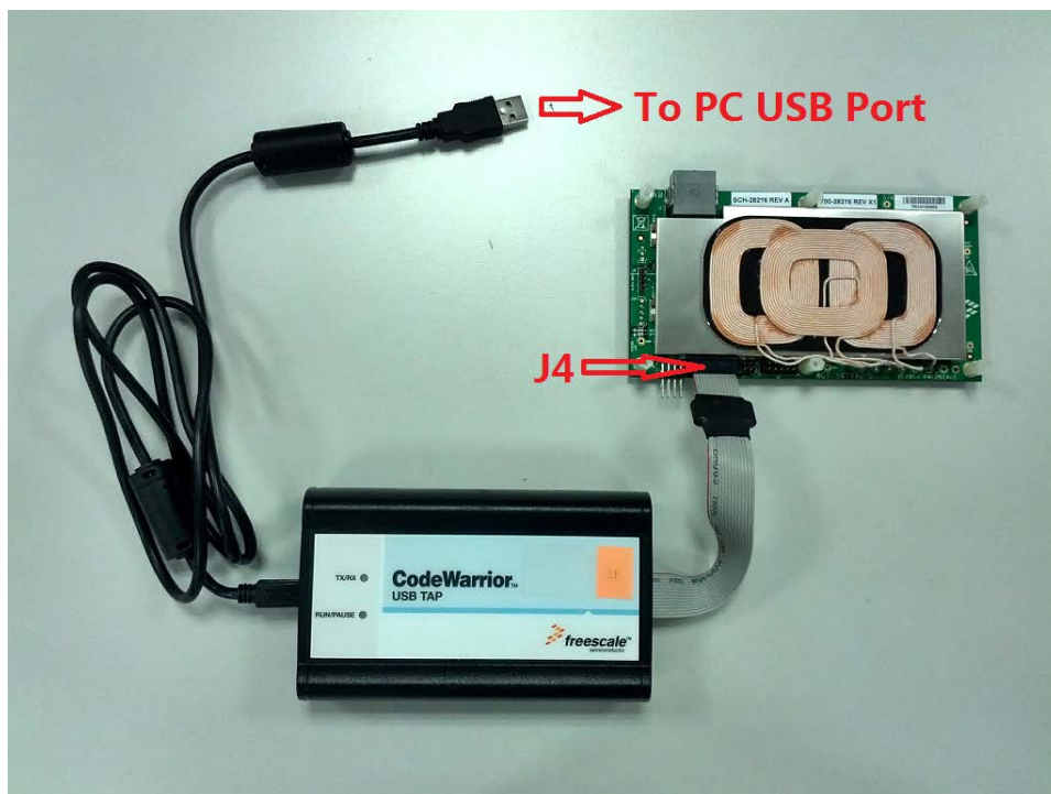
Figure 29 Connecting the debug cable to the board
