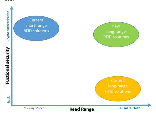
The latest long-range RFID solutions meet the need for high read range plus high security
