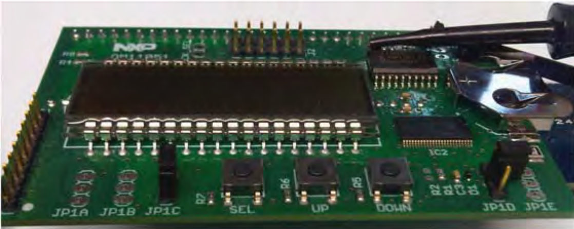
Fig 2. SMD LCD display with fixed pins
